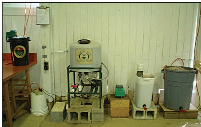
Some examples of commercial and homemade aerated compost tea brewers.
